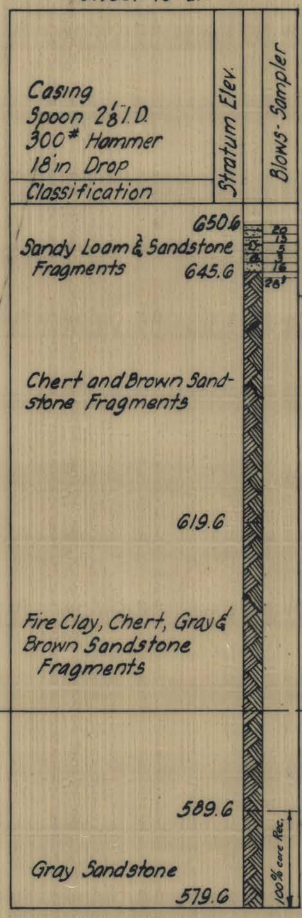
BORING NO. 2L Sta. 10+19 Offset 15 Lt.
