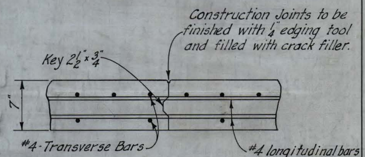
TYPICAL CONSTRUCTION JOINT Scale: 1/2" = 1'-0"
